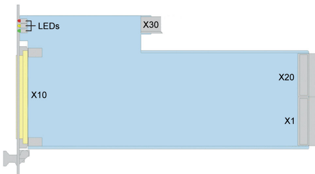
Figure 4-1: Layout of Connectors and LED's
